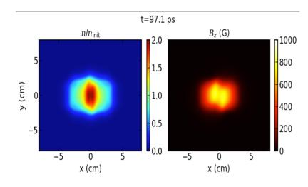
Density and magnetic field of two colliding magnetized plasma jets with parameters relevant to Plasma Liner Experiment at Los Alamos National Lab (credit Han Wen. See also S. Hsu et al IEEE Transaction on Plasma Science 40, 1287 (2012)
